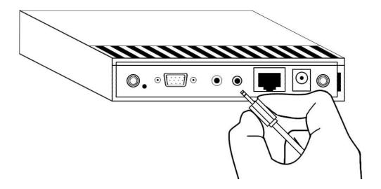
5. Insert VGA cable which connects with external video display to VGA connector located at the back of this projector server.
