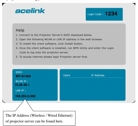
The IP address of the WLAN (wireless Ethernet) and LAN (wired Ethernet) interface of projector server can be found at the lower-left corner of video display. You can use one of these IP addresses to connect to the projector server.
