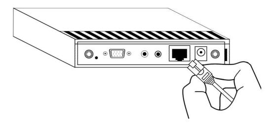
4. Insert the audio cable which connects with external amplifier / speaker to 'Audio Out' port located at the back of this projector server.
