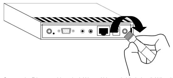
3. Connect the Ethernet cable to the LAN port (this port is labeled as 'LAN' and located at the back of this projector server)
