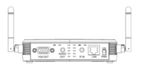
Description Name Connect to A/C adapter / 12V Edimax projector's D/C power outlet 10/100Mbps fast Ethernet LAN port IR IN Connect to IR receiver Audio Out Stereo audio output VGA OUT VGA video output Receives wireless signal. Antenna
