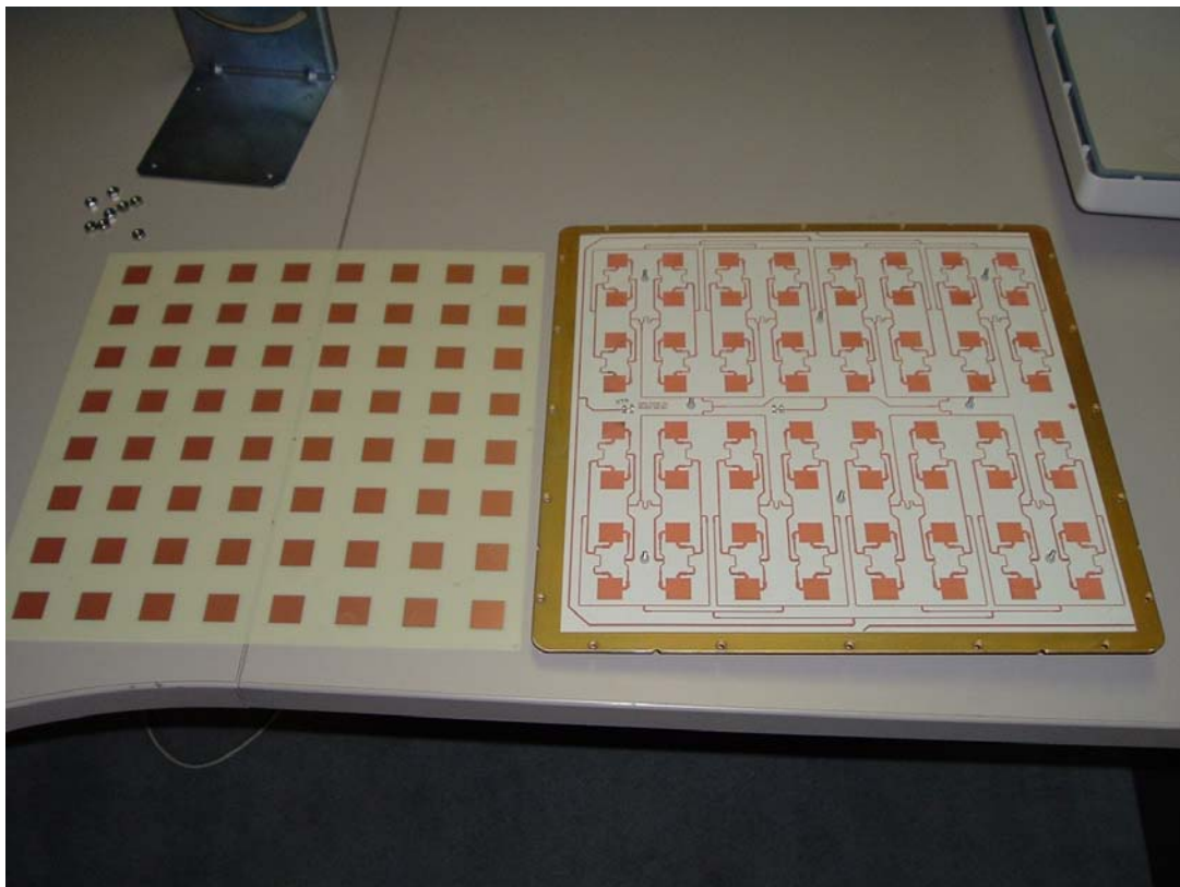
Internal – Inside antenna, parasitic array removed
