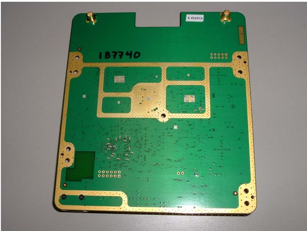
Internal – Back side of radio PCB – Same for all three models
