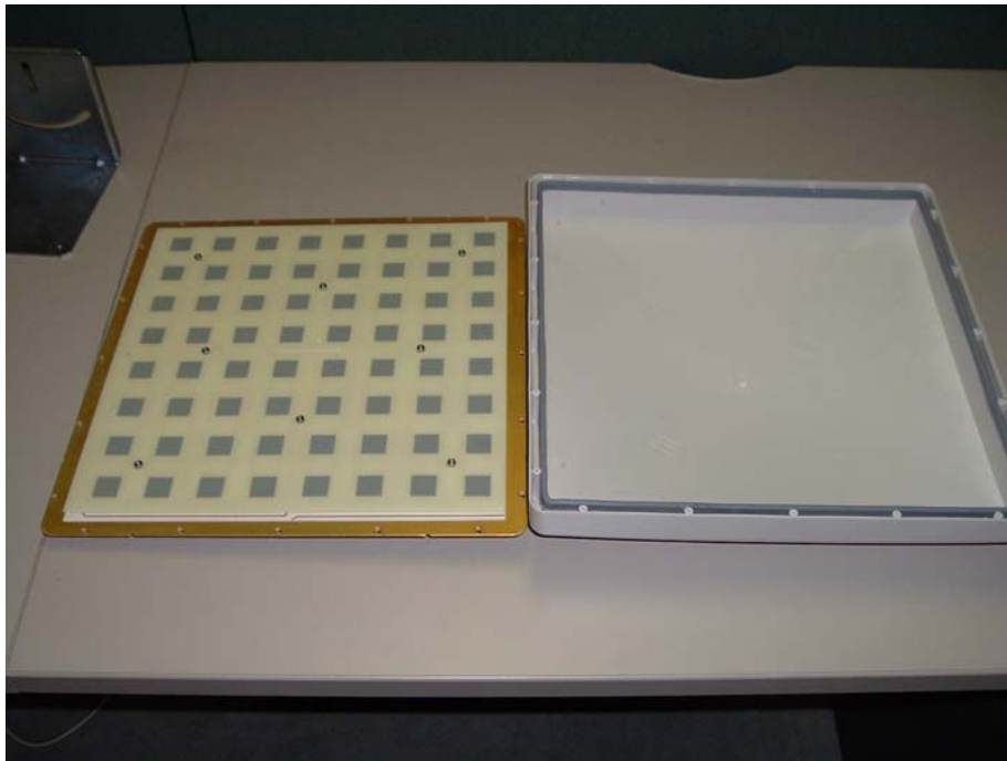
Internal – Inside antenna, radome removed
