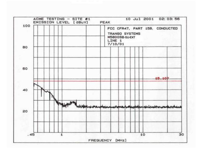
FCC RULES 47CFR PART 15B, SUBPART 15.107,CLASS B CONDUCTED EMISSIONS (0.45 MHZ TO 30 MHZ) 60 Hz/120 VAC LINE 2
