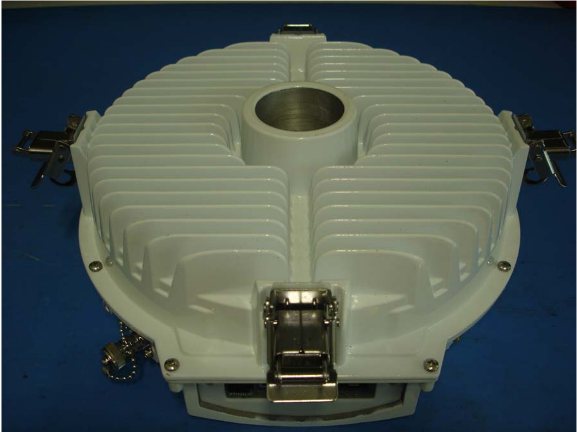
Bottom – Antenna Interface
