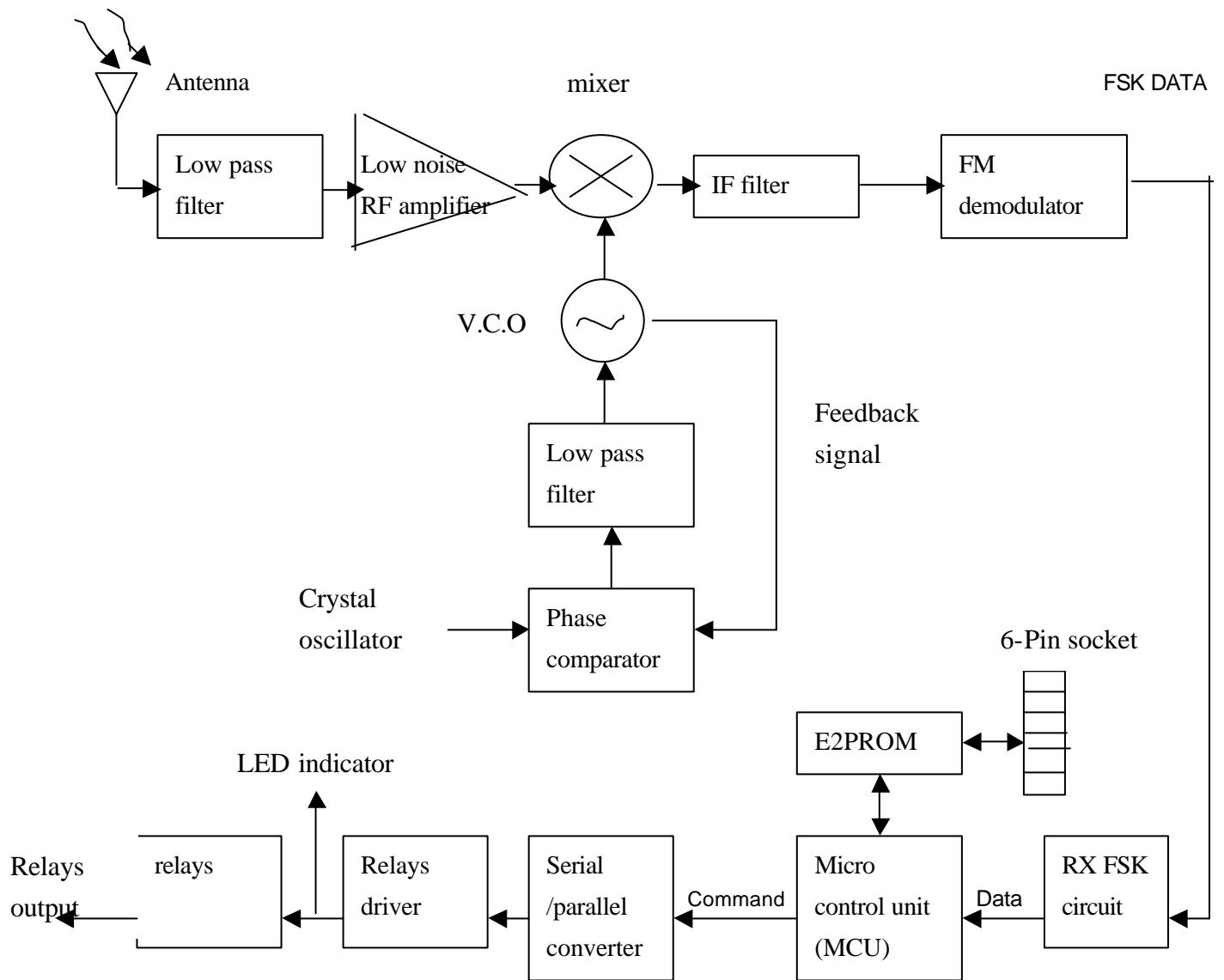
Fig.2 Receiver's function block diagram
