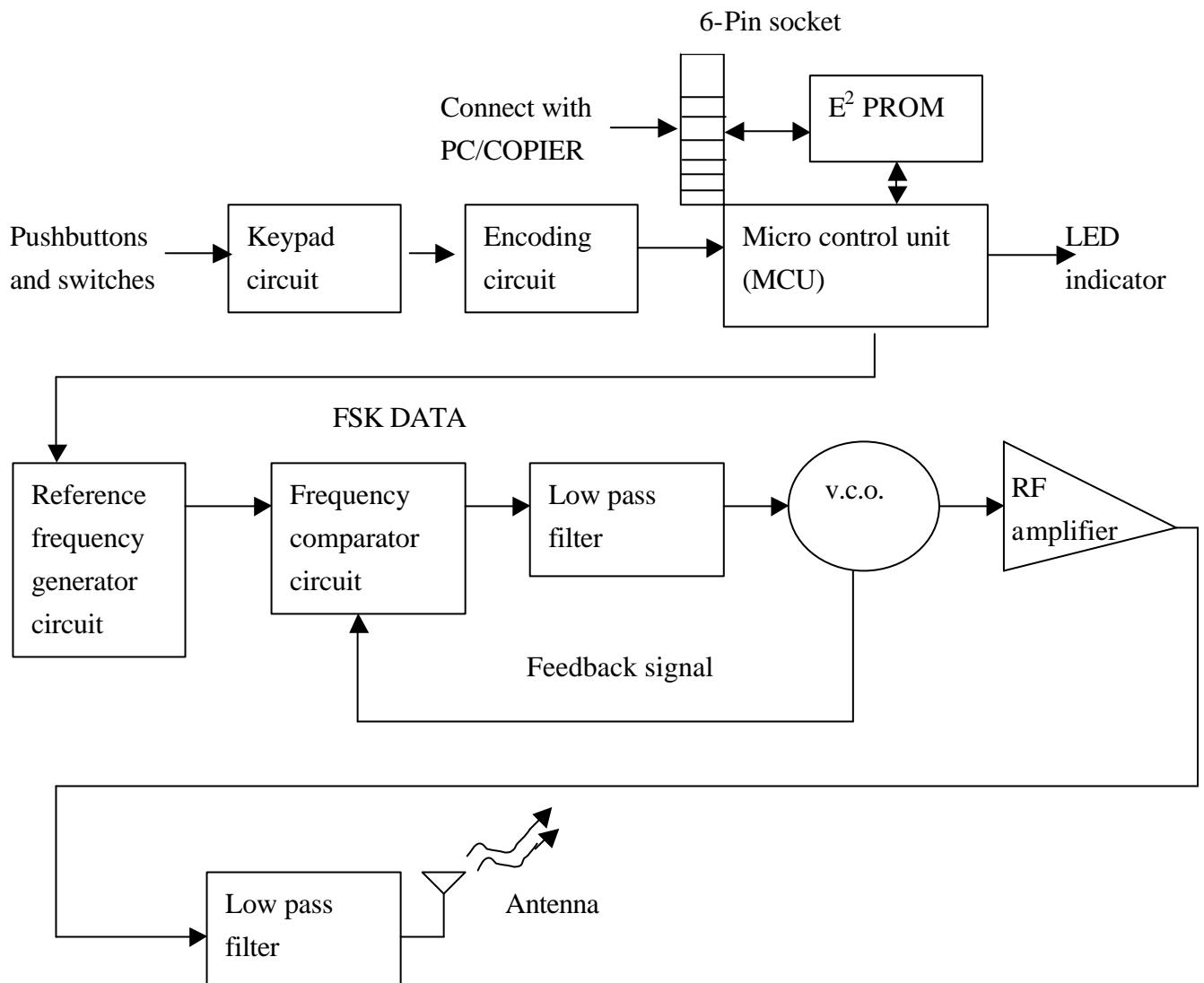
Fig.1 Transmitter' s function block diagram
