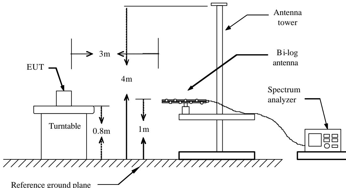
**Above 1 GHz**
