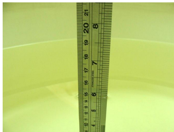
Fig 6.2 Photo of Liquid Height for Body SAR
