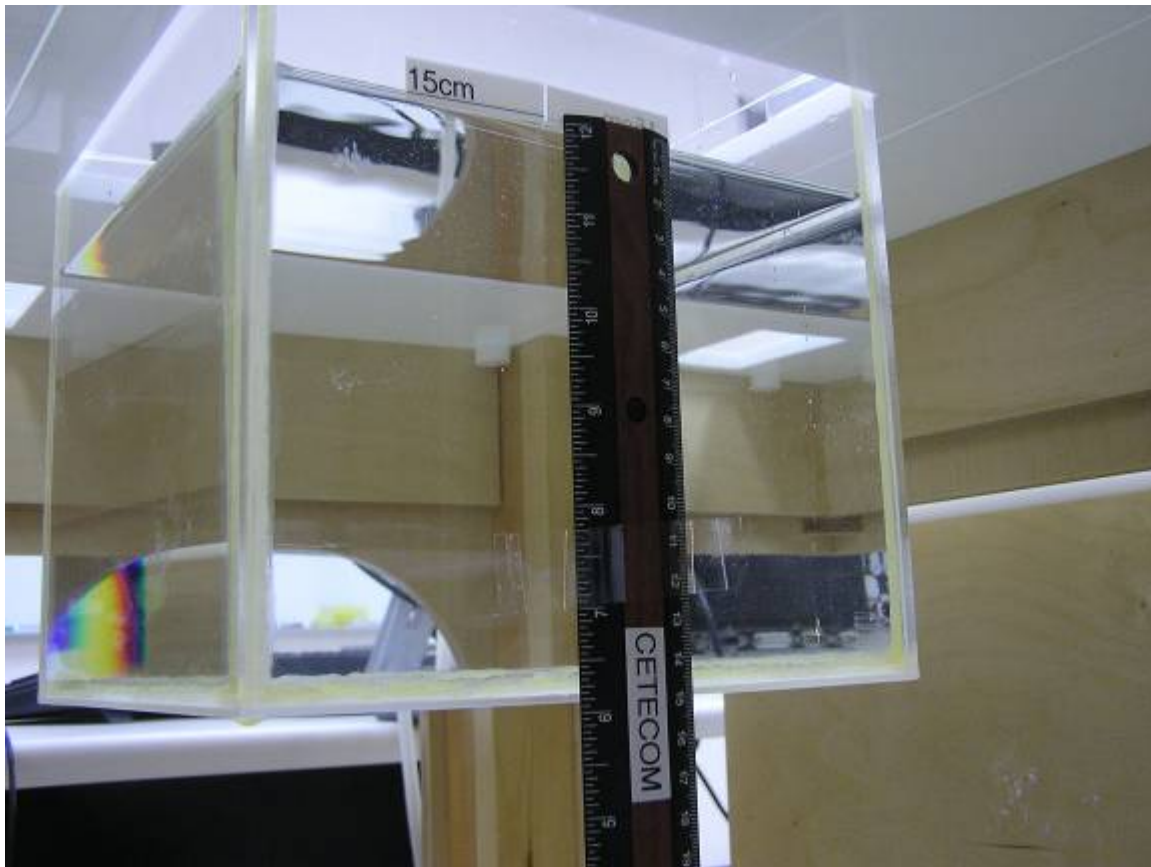
Photo 2. Photo to demonstrate 15 cm Z-axis flat phantom
