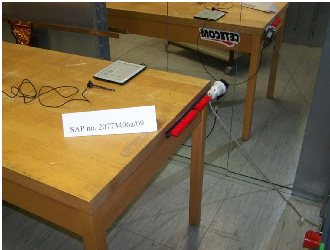
Conducted measurement set-up - emissions generated on AC-mains
