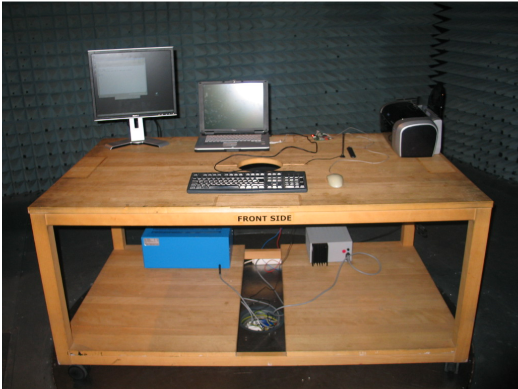
Photo 2: Test setup for radiated measurements
