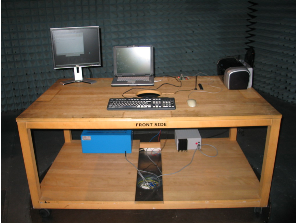
Photo 2: Test setup for radiated measurements
