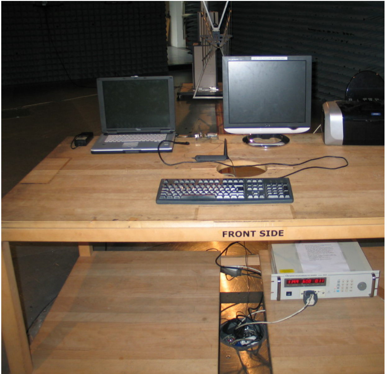
set-up for radiated tests
