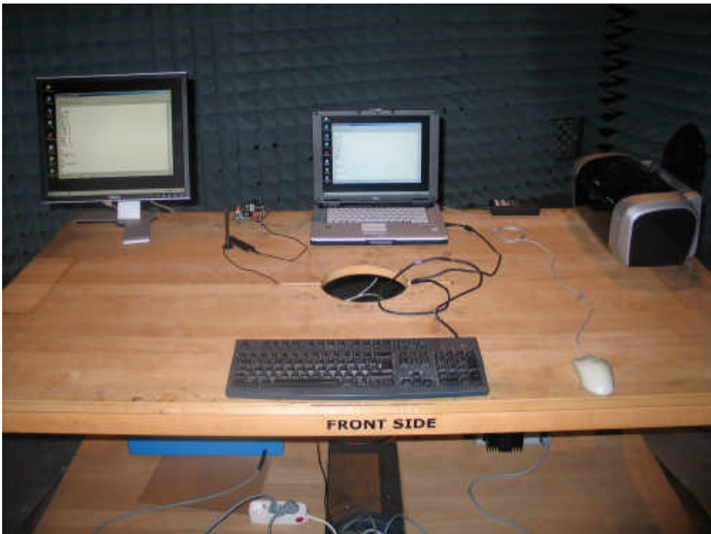
Photo 2: Test setup for radiated measurements
