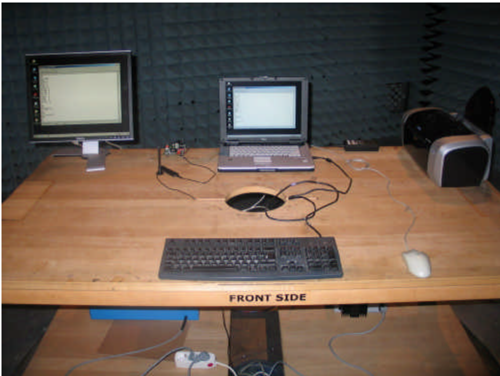
Photo 2: Test setup for radiated measurements
