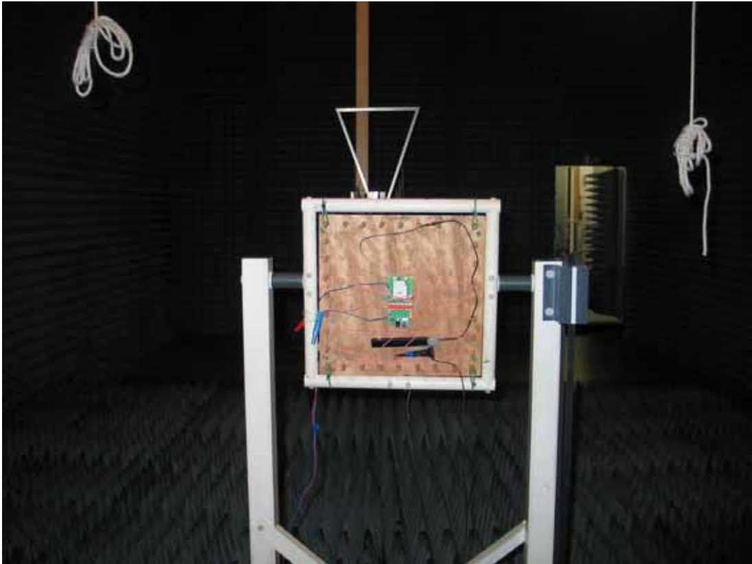
Photo 4: Setup for radiated tests (EUT operated in a cradle and with external antenna)
