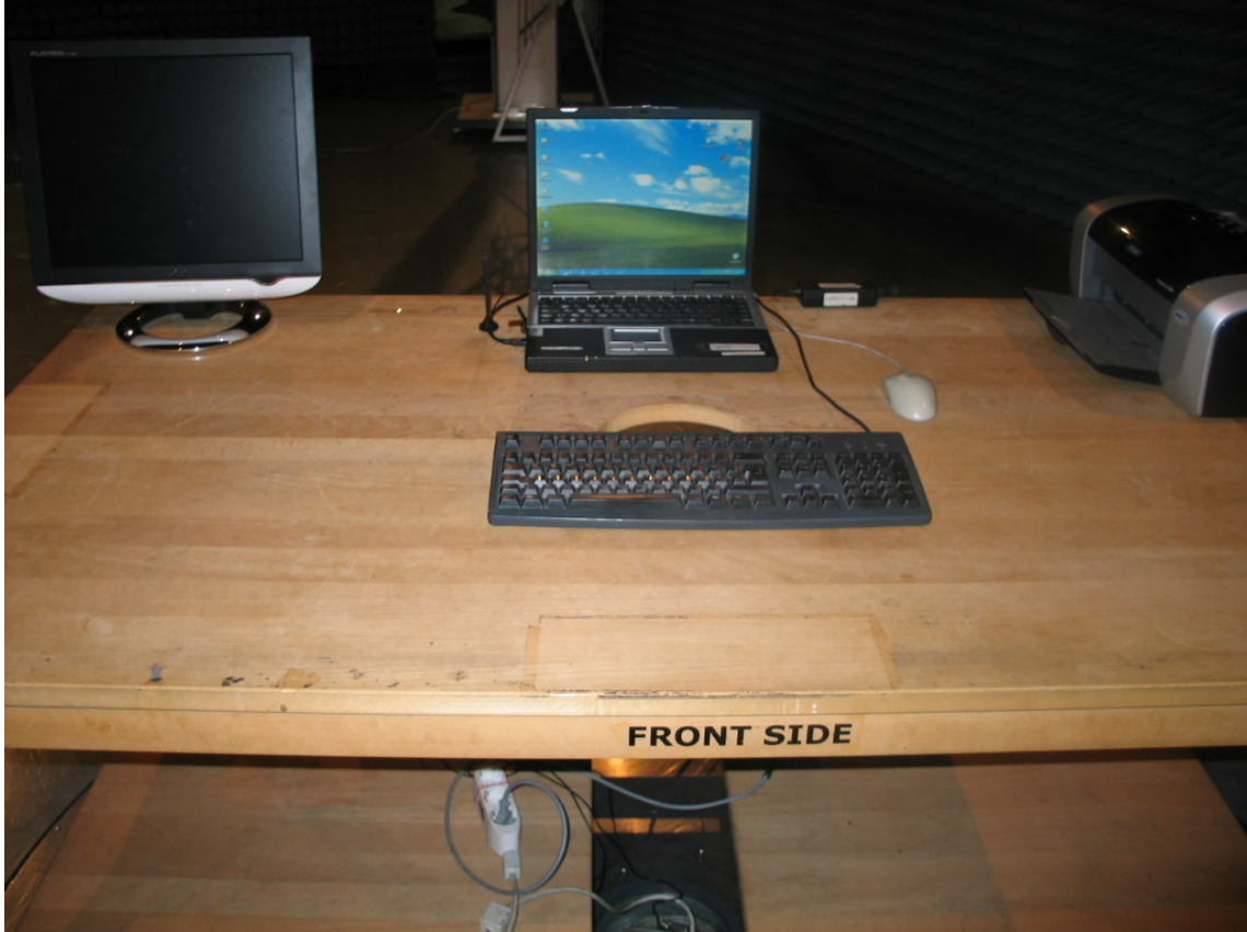
Photo 1: Test setup for radiated measurements
