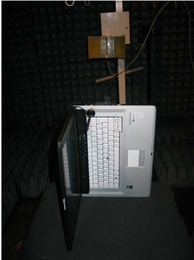
Photo 3: Test setup a01 in the anechoic chamber
