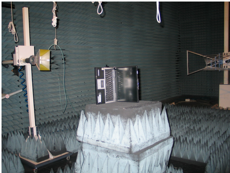
Photo 4: Test setup b01 in the anechoic chamber
