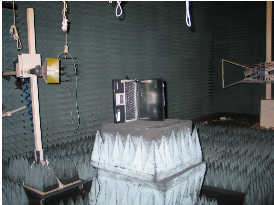
Photo 4: Test setup b01 in the anechoic chamber
