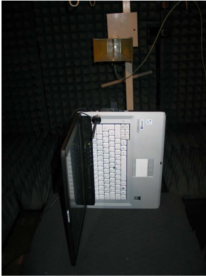
Photo 3: Test setup a01 in the anechoic chamber
