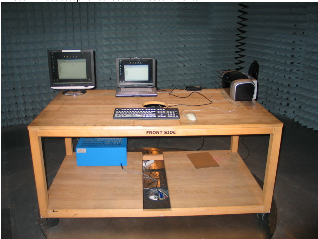
Photo 2: Test setup for radiated measurements
