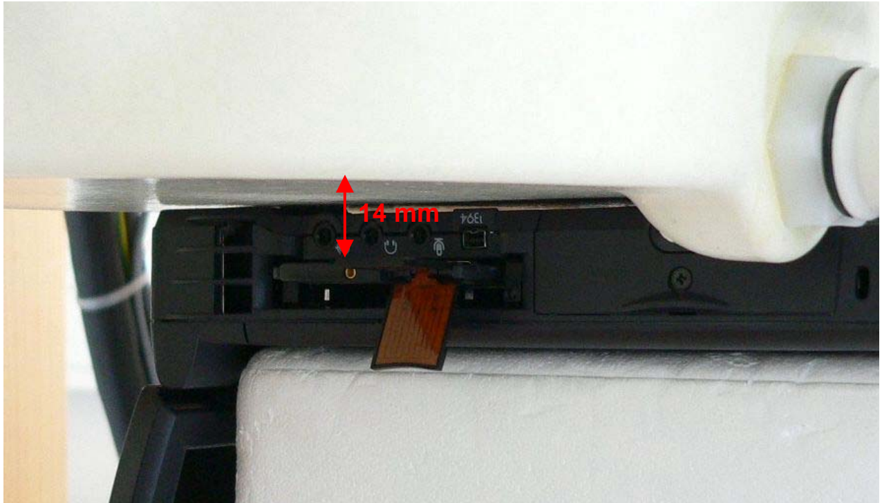
Fig. 24: Lap Held Position with the DELL Latitude C810 Notebook, antenna in intended use position.
