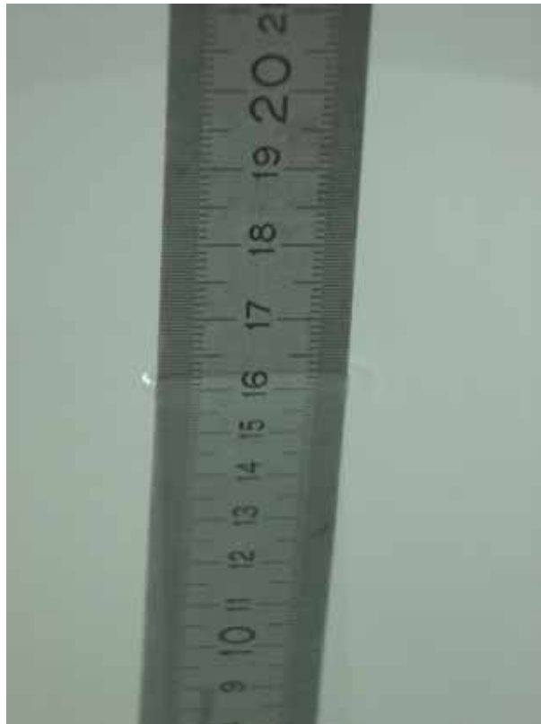
Fig. 28: Liquid depth for GPRS 1900 Body measurements.
