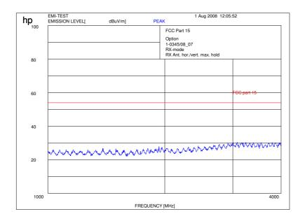
f < 1 GHz: RBW / VBW: 100 kHz  $f \ge 1 \text{GHz}: \text{RBW / VBW}: 1 \text{ MHz}$
