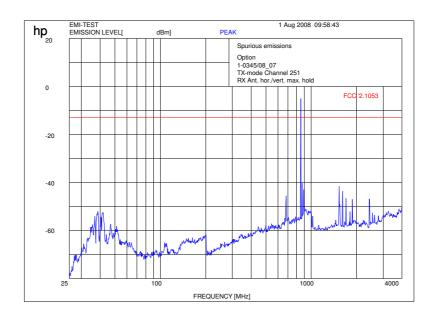
f < 1 GHz: RBW / VBW: 100 kHz  $f \ge 1 \text{GHz}$ : RBW / VBW: 1 MHz
