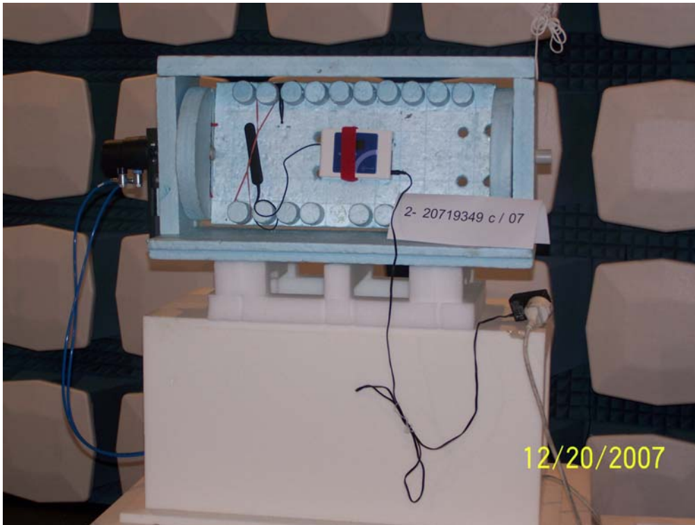
Photograph 5: Measurements in the anechoic chamber: Test Set-up
