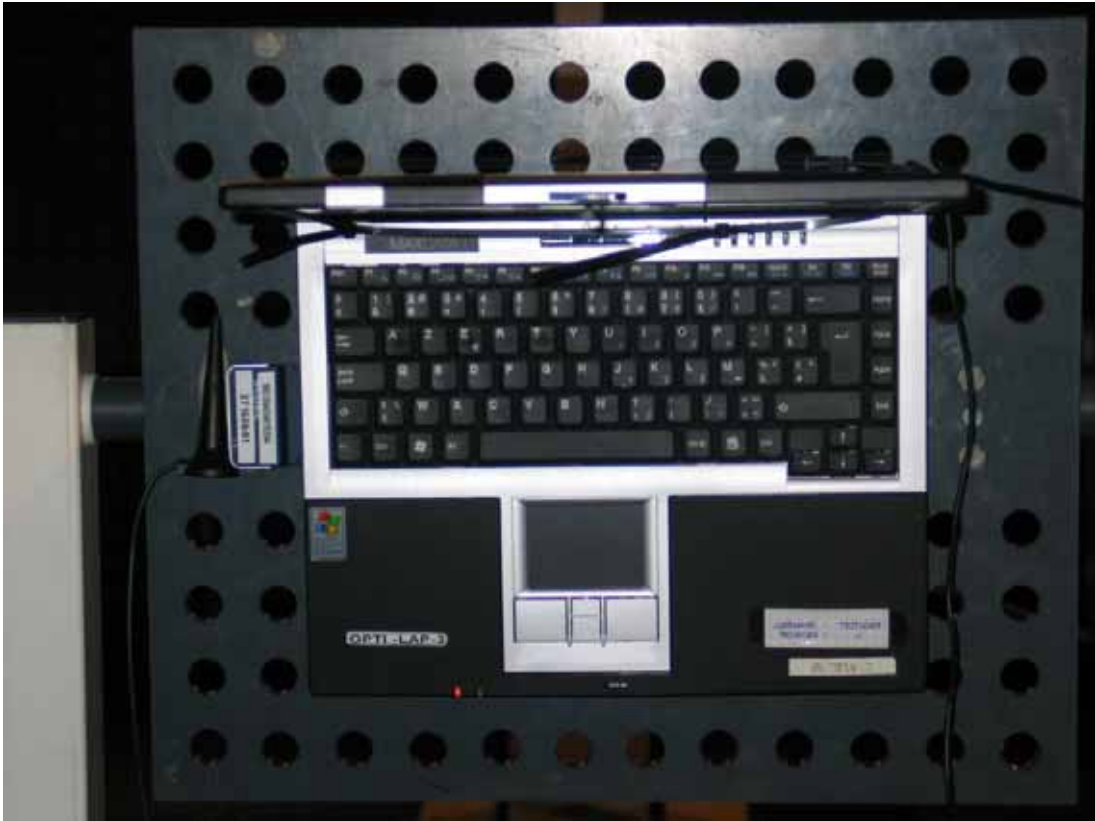
Photo 4: Setup for radiated tests
