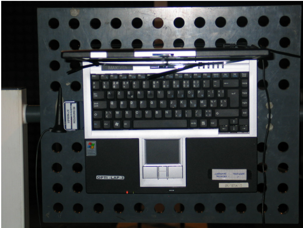
Photo 4: Setup for radiated tests
