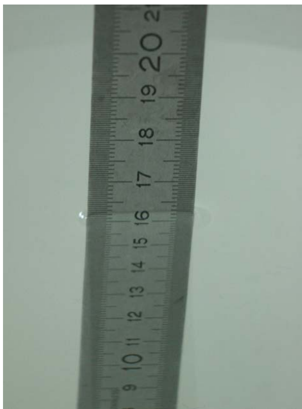
Fig. 26: Liquid depth for GPRS 1900 Body measurements.
