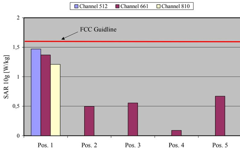
Fig. 13: The measured SAR values for the Option Fusion Quad Band Card in combination with an ACER Aspire 2020 Notebook for GPRS 1900 in comparison to the FCC exposure limit.
