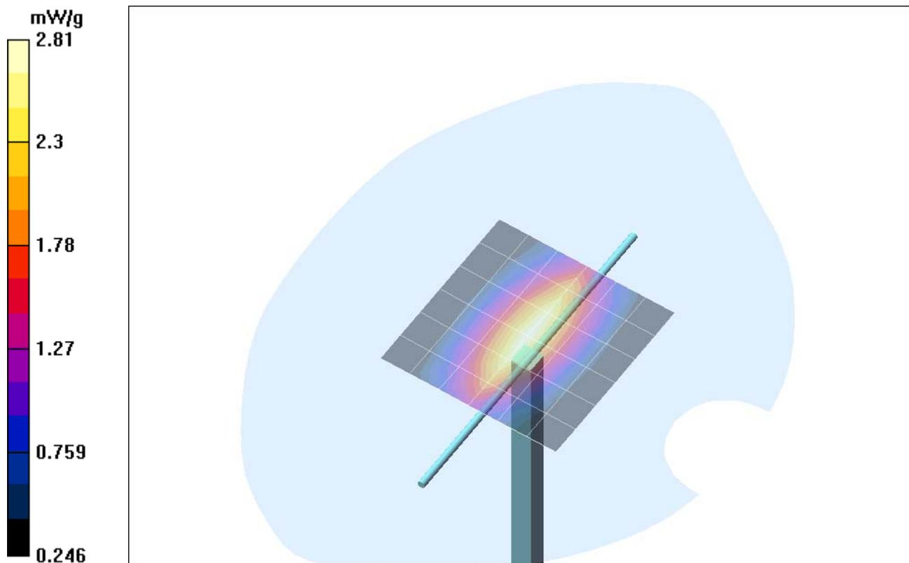
Fig. 14: Validation measurement 835MHz Body (November 25, 2004), coarse grid.
