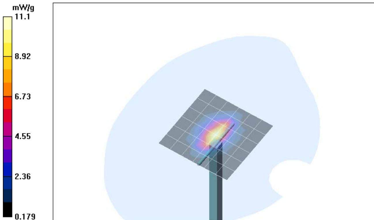
Fig. 16: Validation measurement 1900 MHz Body (November 24, 2004), coarse grid.
