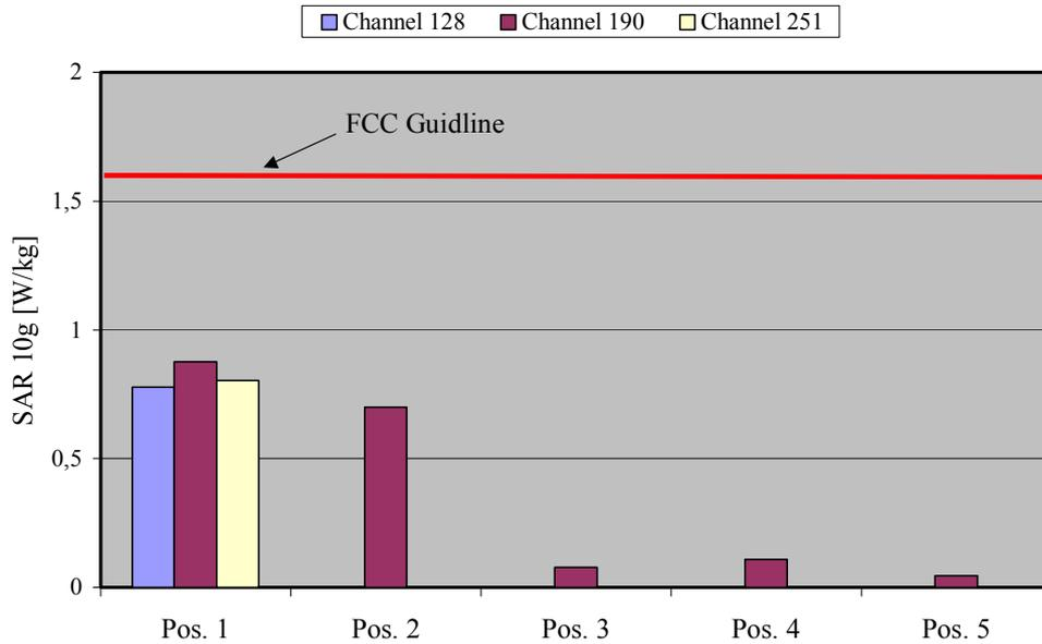
Fig. 8: The measured SAR values for the Option Fusion Quad Band Card in combination with a DELL Latitude D505 Notebook for GPRS 850 in comparison to the FCC exposure limit.
