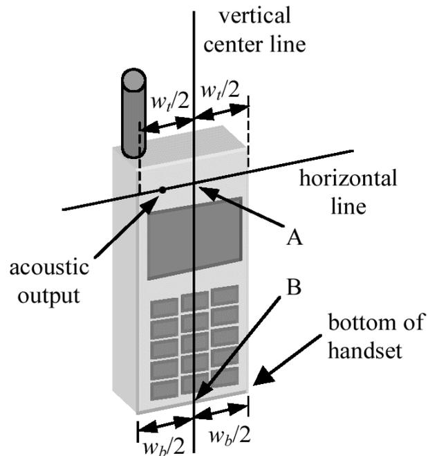
Fig. 2: Handset vertical and horizontal reference lines.
