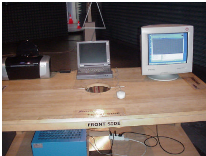
Picture 2: Setup for radiated measurements below 1 GHz
