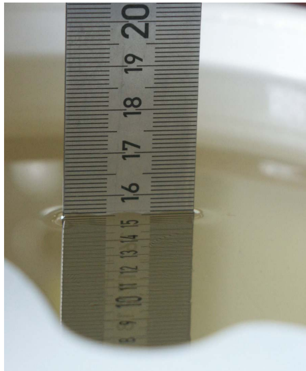
Fig. 24: Liquid depth for GSM 850 Body measurements.
