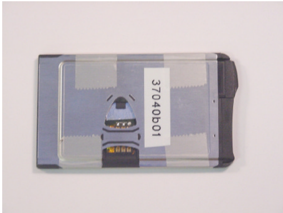
Picture 1 : EUT (topside, with antenna connector for radiated measurements)
