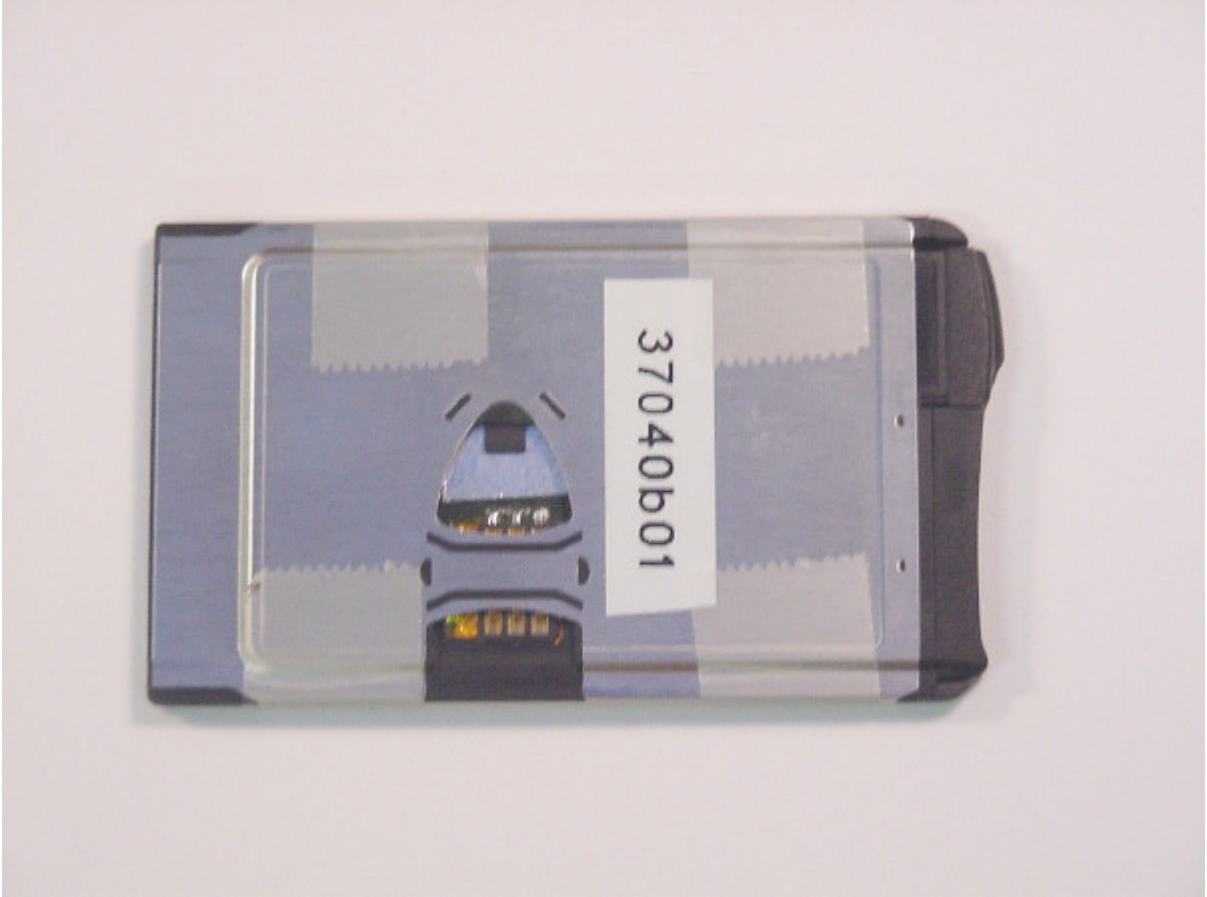
Photo 1: EUT (topside, with antenna connector for radiated measurements)
