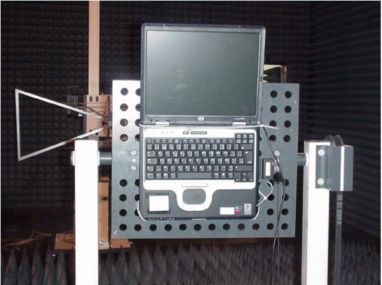
Photo 3: Setup for radiated tests
