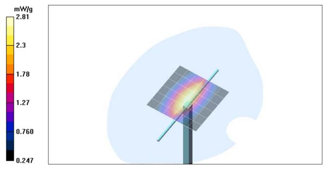
Fig. 15: Validation measurement 835MHz Body (November 29, 2004), coarse grid. Ambient Temperature: 22.0° C, Liquid Temperature: 21.0° C.
