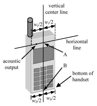
Fig. 2: Handset vertical and horizontal reference lines.
