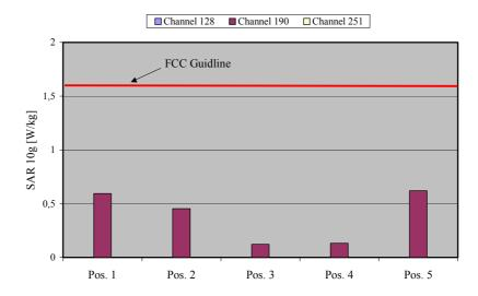
Fig. 9: The measured SAR values for the Option Fusion Quad Band Card in combination with a Packard Bell Easy Note Notebook for GPRS 850 in comparison to the FCC exposure limit.
