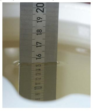
Fig. 36: Liquid depth for GPRS 850 Body measurements.
