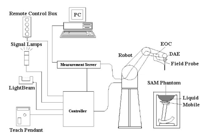
Fig. 6: The DASY4 measurement system.
