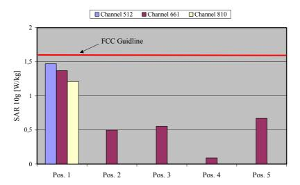
Fig. 13: The measured SAR values for the Option Fusion Quad Band Card in combination with a ACER Aspire 2020 Notebook for GPRS 1900 in comparison to the FCC exposure limit.
