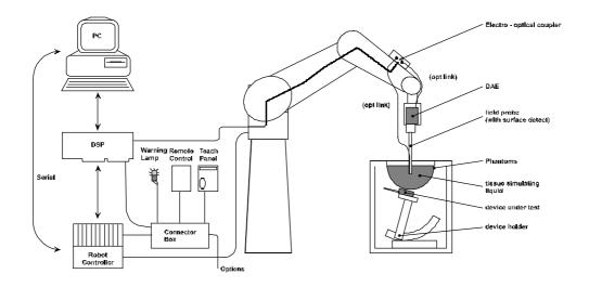
The DASY3 system for performing compliance tests consist of the following items:
