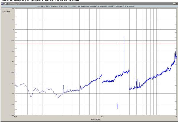
Test: 24.4; Frequency Band = FDD2, Mode = HSDPA, Channel = 9400, Frequency = 1880MHz
