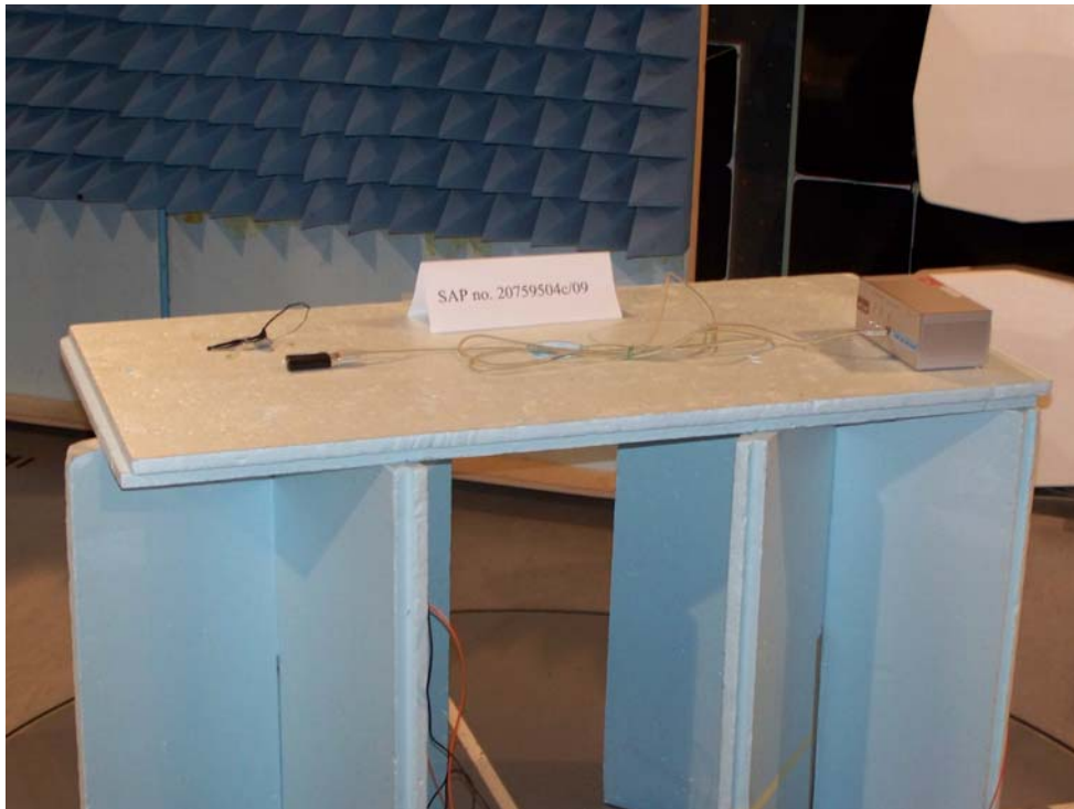
Photograph 1: SET-up radiated tests
