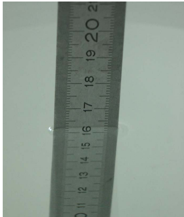
Fig. 26: Liquid depth for GPRS 1900 and WCDMA II Body measurements.
