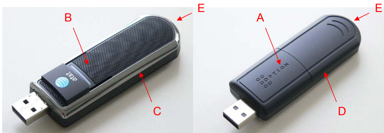
Fig. 3: Device under the test: Option GI0461 with all applicable orientations.
