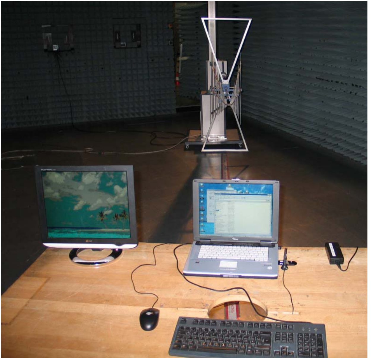
set-up for radiated tests
