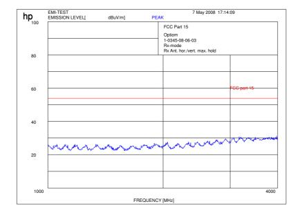
f < 1 GHz : RBW/VBW: 100 kHz  $f \ge 1 \text{GHz}: \text{RBW / VBW 1 MHz}$
