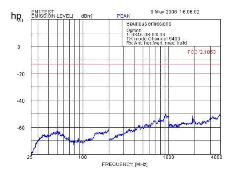
f < 1 GHz : RBW/VBW: 100 kHz Carrier suppressed with a rejection filter
