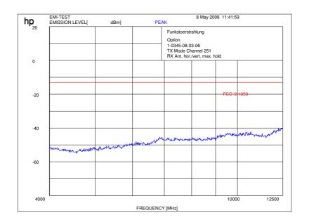
f < 1 GHz: RBW/VBW: 100 kHz  $f \ge 1 \text{ GHz}: RBW / VBW 1 \text{ MHz}$
