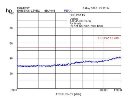
f < 1 GHz: RBW/VBW: 100 kHz  $f \ge 1 \text{ GHz}: RBW / VBW 1 \text{ MHz}$
