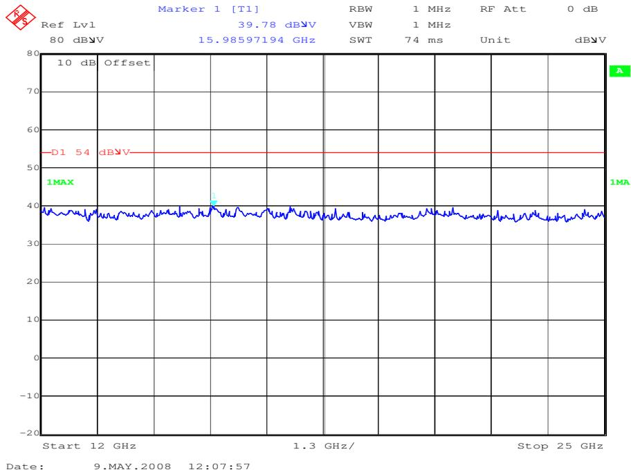
**Measurement Results: Radiated Emissions with 3<sup>rd</sup> Laptop – Fujitsu/Siemens AmiloPro (SPQ-Testunit-193)**
