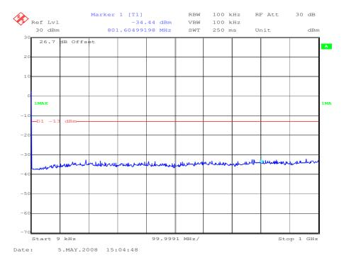
The peak at the beginning of the Plot is the LO from the measuring spectrum Analyzer and not from the EUT
