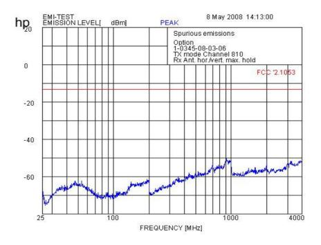
f < 1 GHz : RBW/VBW: 100 kHz Carrier suppressed with a rejection filter
