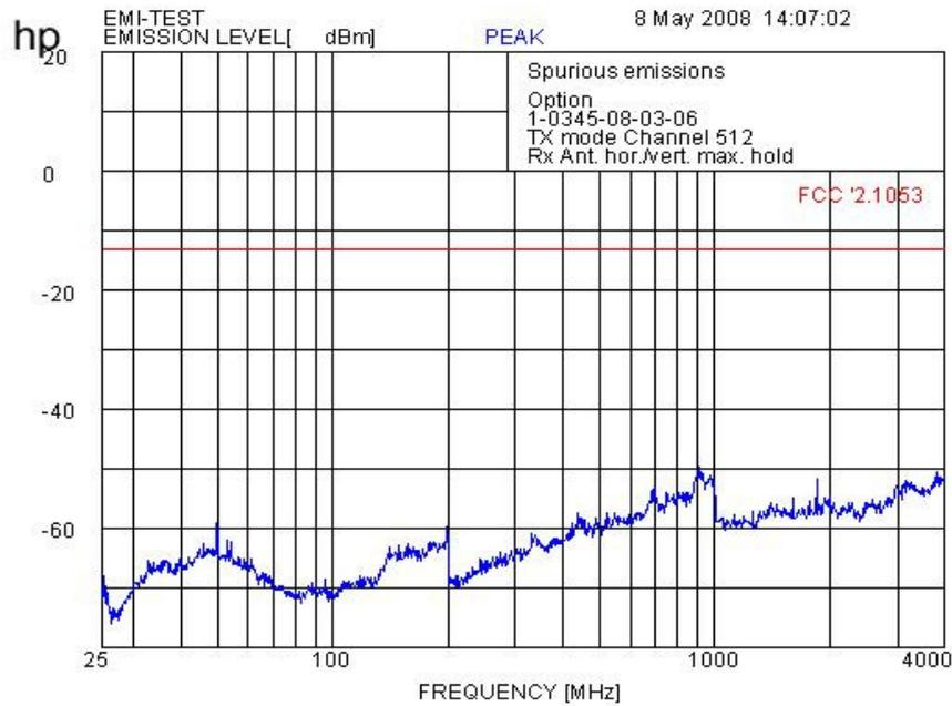
f < 1 GHz : RBW/VBW: 100 kHz      f ≥ 1GHz : RBW / VBW 1 MHz
