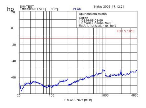
f < 1 GHz : RBW/VBW: 100 kHz Carrier suppressed with a rejection filter f > 1 GHz : RBW / VBW 1 MHz
