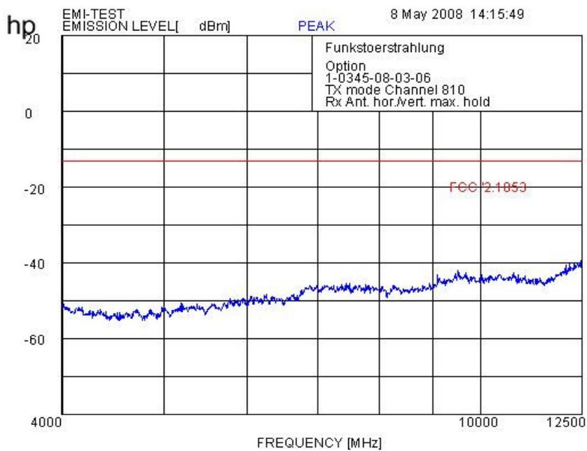
f < 1 GHz : RBW/VBW: 100 kHz      f ≥ 1GHz : RBW / VBW 1 MHz
