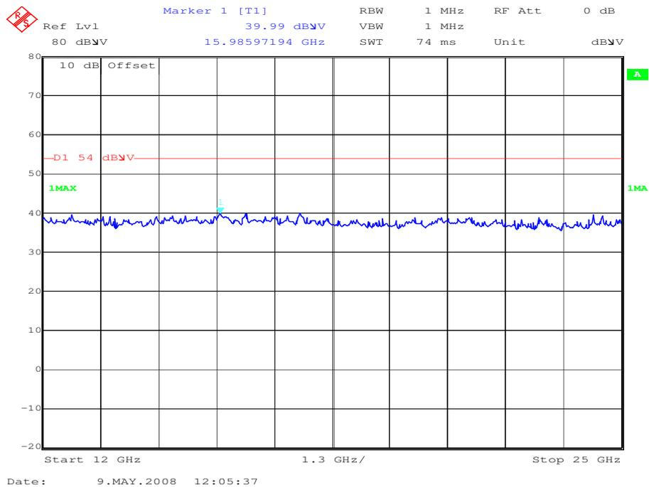
**Measurement Results: Radiated Emissions with 2<sup>nd</sup> Laptop – DELL PP01X (SPQ-Testunit-47)**
