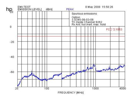
f < 1 GHz : RBW/VBW: 100 kHz Carrier suppressed with a rejection filter f > 1 GHz: RBW / VBW 1 MHz
