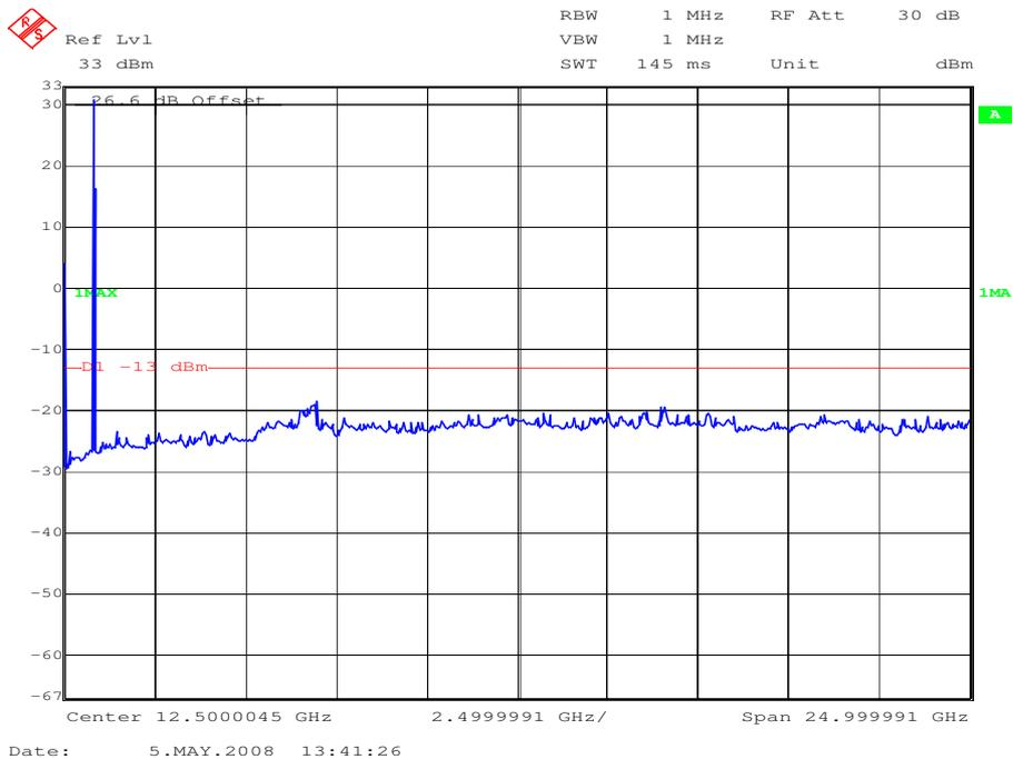
*The peak at the beginning of the Plot is the LO from the measuring spectrum Analyzer and not from the EUT.*
