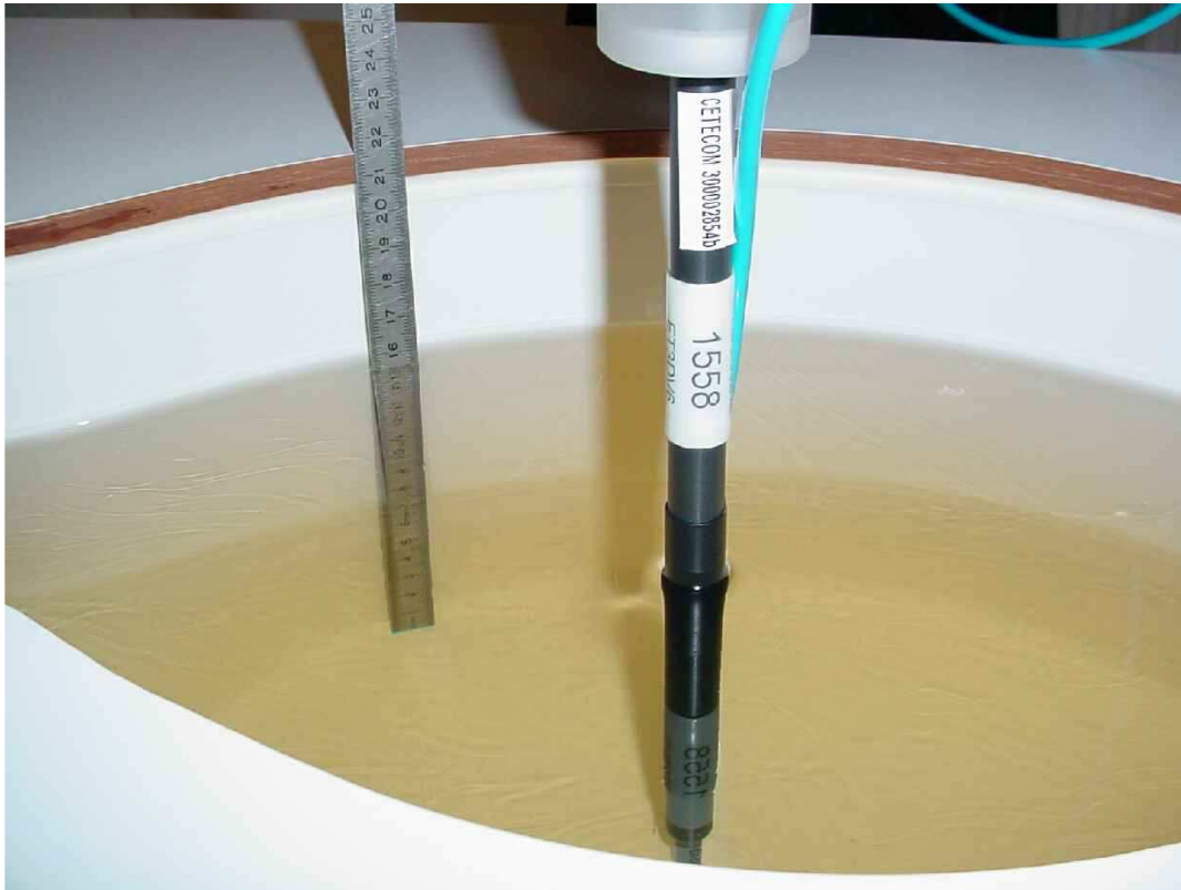
Photo 26: Liquid depth 1900 MHz body simulating liquid
