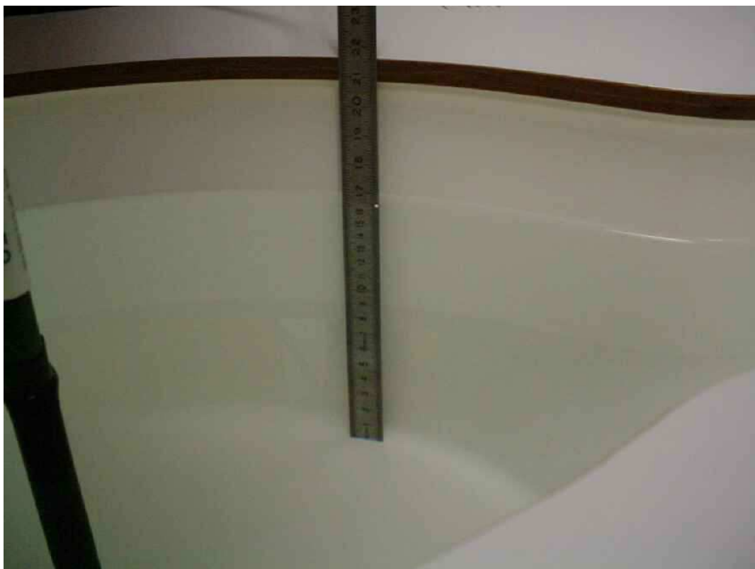
Photo 26: Liquid depth 1900 MHz body simulating liquid
