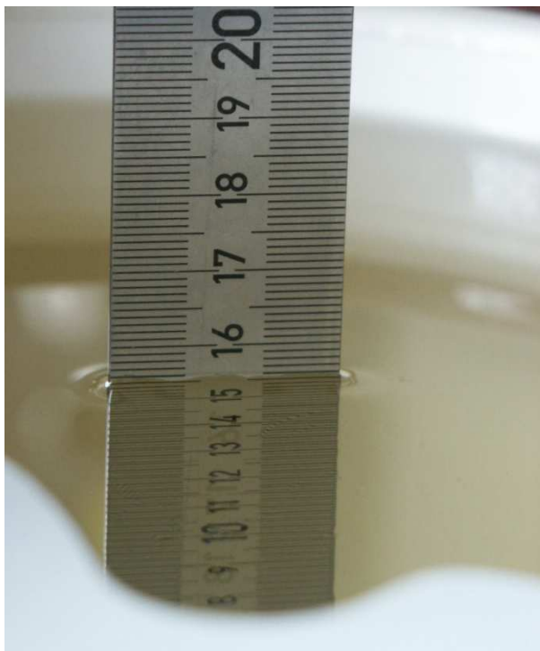
Fig.10.15: Liquid depth for GPRS/EDGE 850 and WCDMA V Body measurements.
