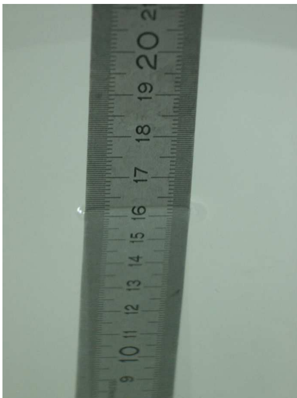
Fig.10.16: Liquid depth for GPRS/EDGE 1900 and WCDMA II Body measurements.
