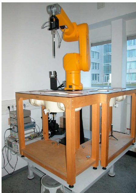
Fig. 6.2: Picture of DASY measurement set-up with SAM Phantom
