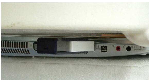
Fig. 4.4: Orientation 2 (Distance DUT «» phantom = 1/2 inch or 5mm)
