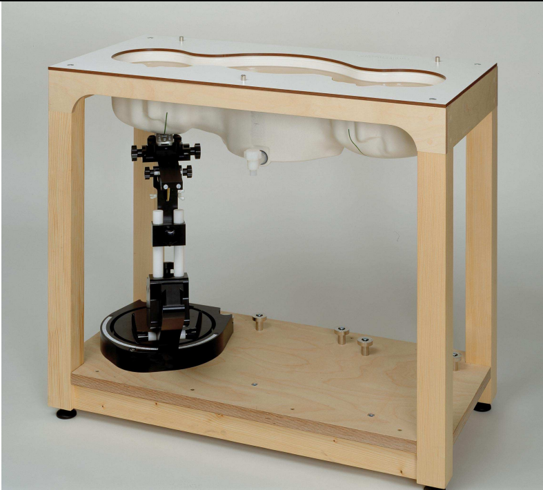
Fig. 6.3: SAM Twin Phantom
