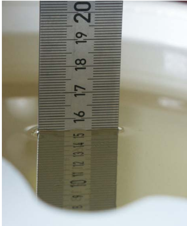
Fig. 26: Liquid depth for GPRS 850 and WCDMA V Body measurements.
