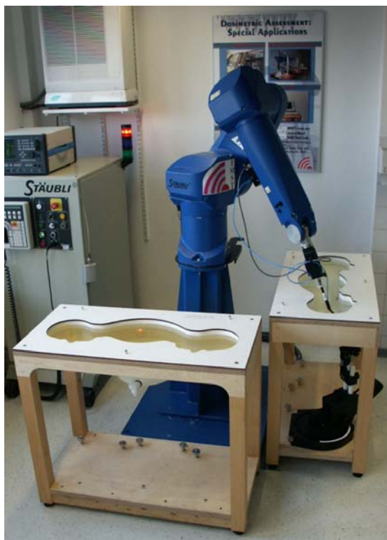
Fig. 6: The measurement set-up with two SAM phantoms containing tissue simulating liquid.
