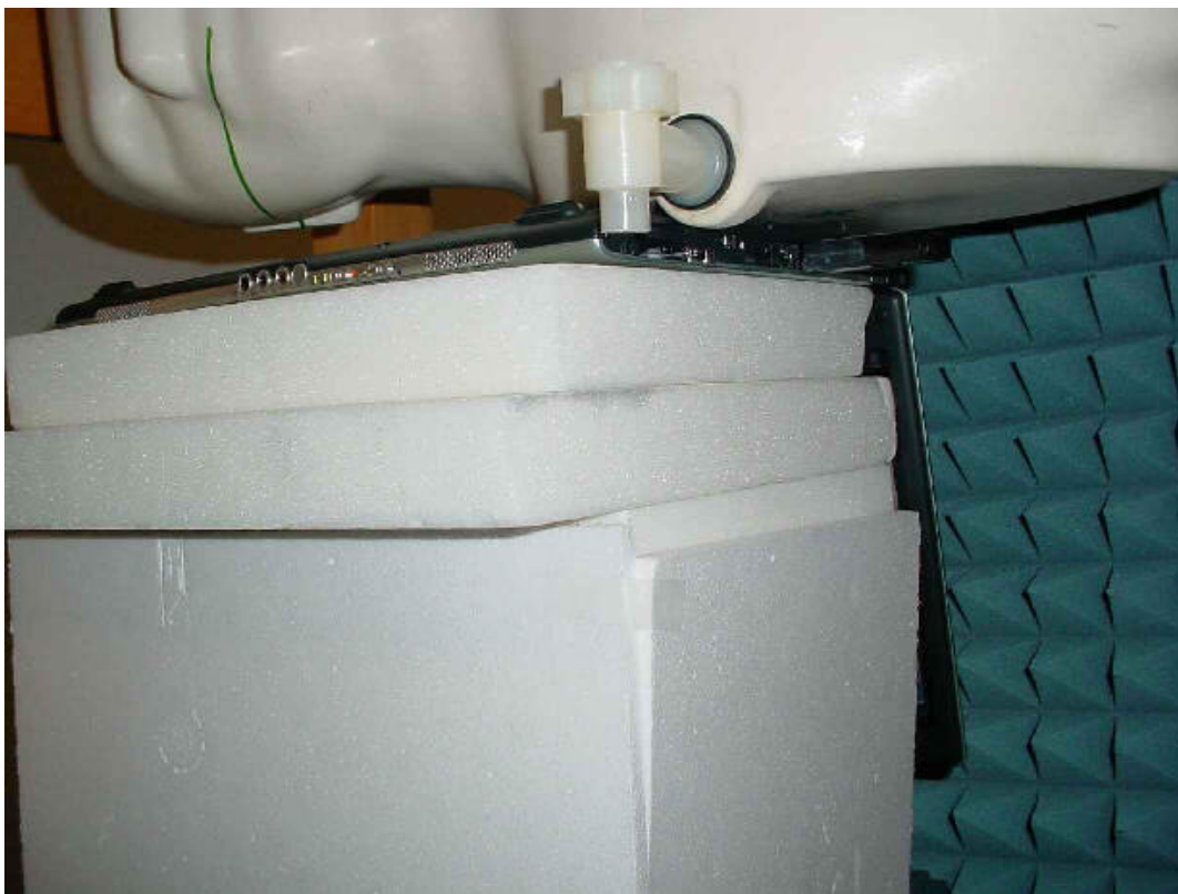
Photo 26: Test position underside with 3rd laptop ( distance 12 mm)
