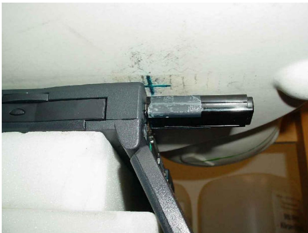
Photo 24: Test position underside with 2nd laptop ( distance 11 mm)
