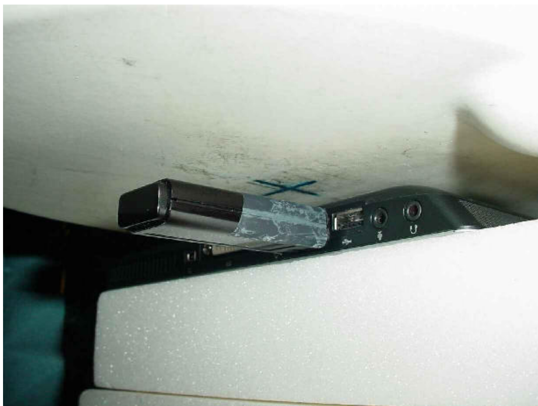
Photo 20: Test position underside with 1st laptop ( distance 10 mm)
