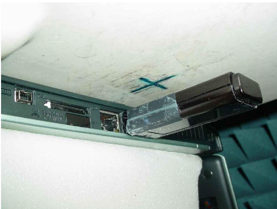
Photo 26: Test position underside with 3rd laptop ( distance 12 mm)
