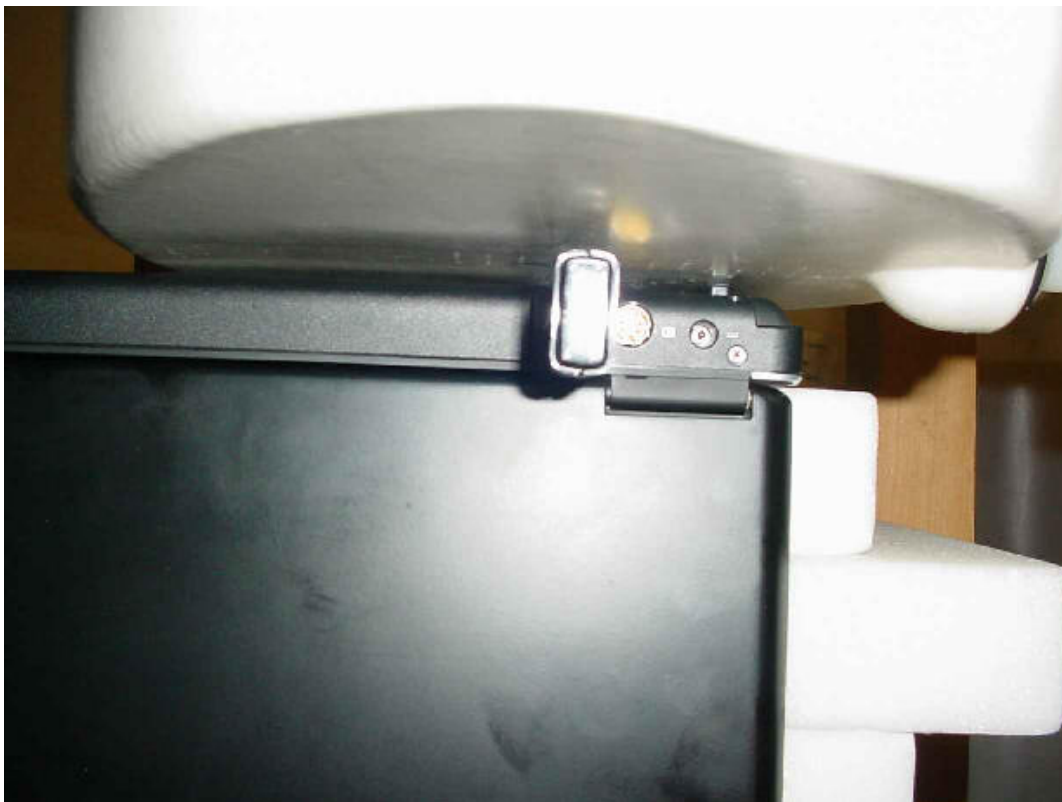
Photo 22: Test position underside with 1st laptop (distance 3 mm) in vertical USB-slot
