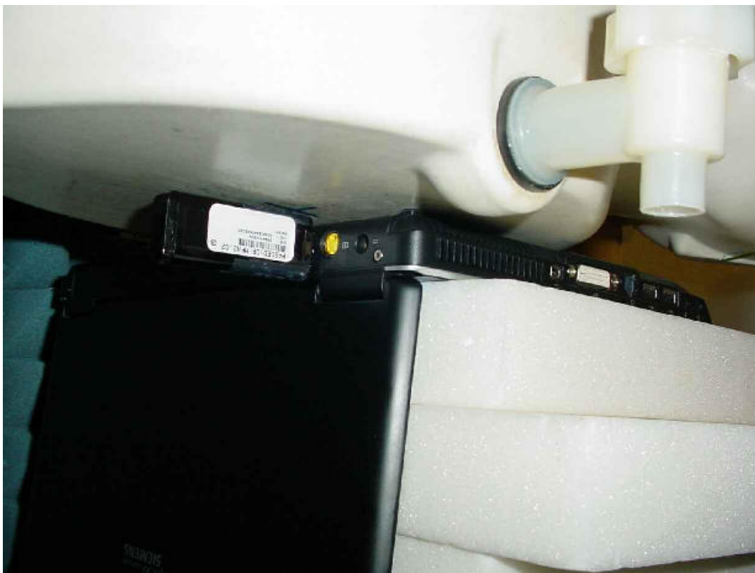
Photo 22: Test position underside with 1st laptop (distance 3 mm) in vertical USB-slot
