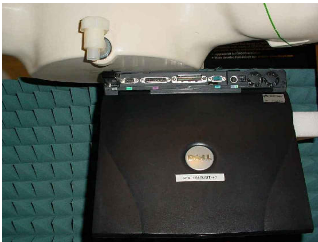
Photo 24: Test position underside with 2nd laptop ( distance 11 mm)
