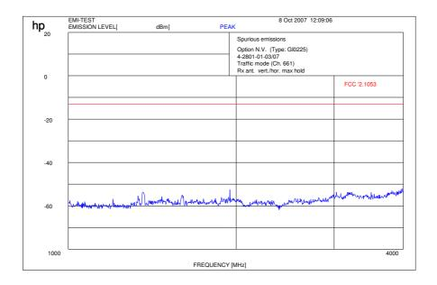
f < 1 GHz: RBW/VBW: 100 kHz  $f \ge 1 \text{GHz}: RBW / VBW 1 \text{ MHz}$  Carrier suppressed with a rejection filter
