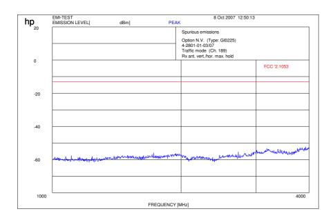
$f < 1 \ GHz : RBW/VBW : 100 \ kHz$   $f \ge 1 GHz : RBW / VBW 1 \ MHz$  Carrier suppressed with a rejection filter
