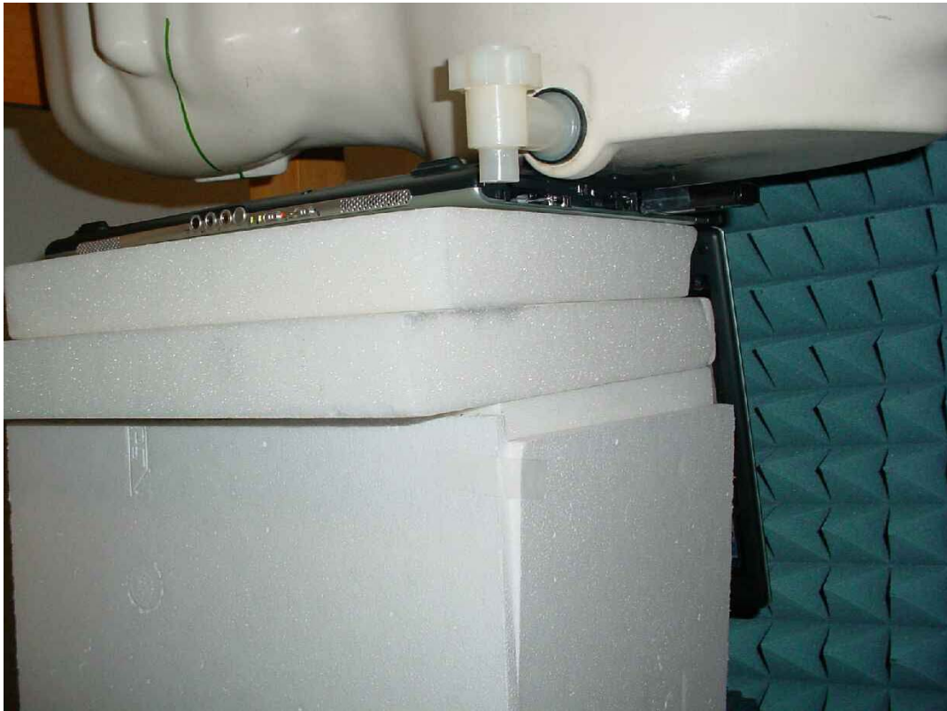
Photo 24: Test position underside with 3rd laptop ( distance 12 mm)
