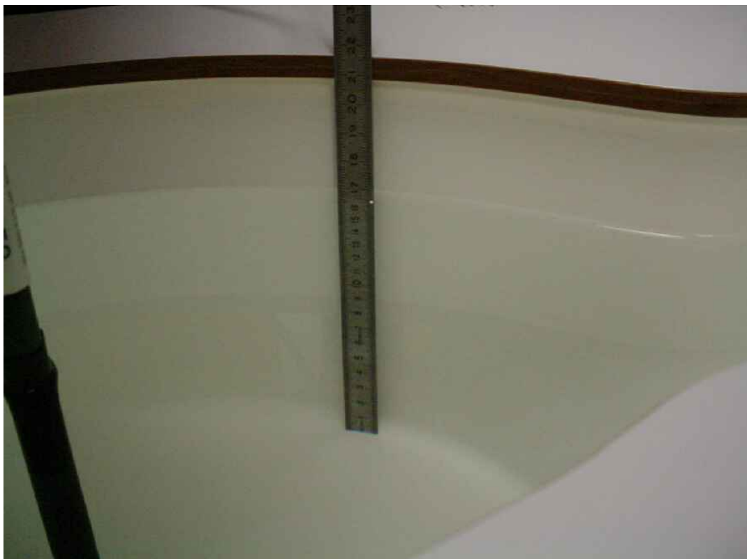
Photo 28: Liquid depth 1900 MHz body simulating liquid
