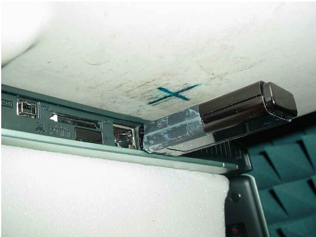
Photo 24: Test position underside with 3rd laptop ( distance 12 mm)
