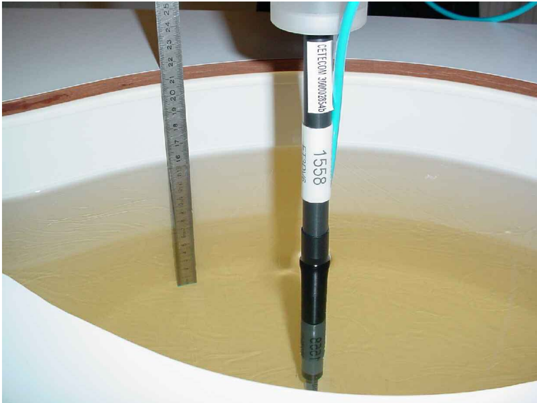
Photo 28: Liquid depth 1900 MHz body simulating liquid
