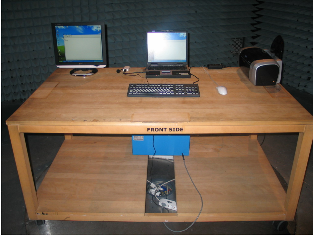
Photo 1: Test setup for radiated measurements
