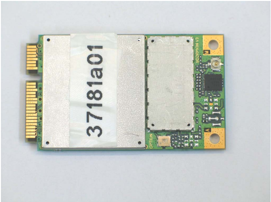
Photo 5: GSM/UMTS module MO0205 (front side)
