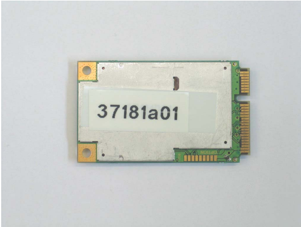
Photo 6: GSM/UMTS module MO0205 (rear side)
