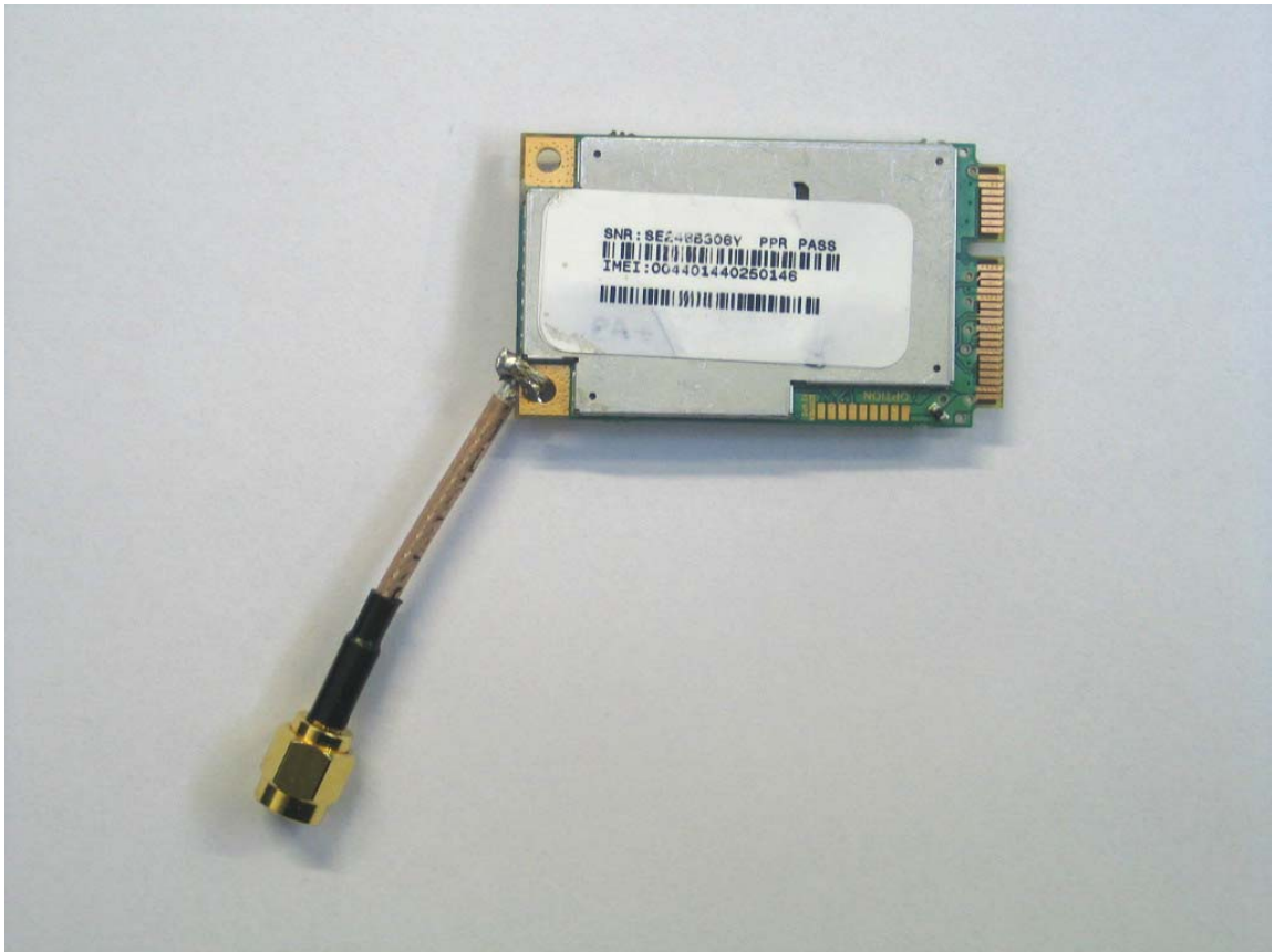
Photo 4: GSM/UMTS module MO0201 (rear side)
