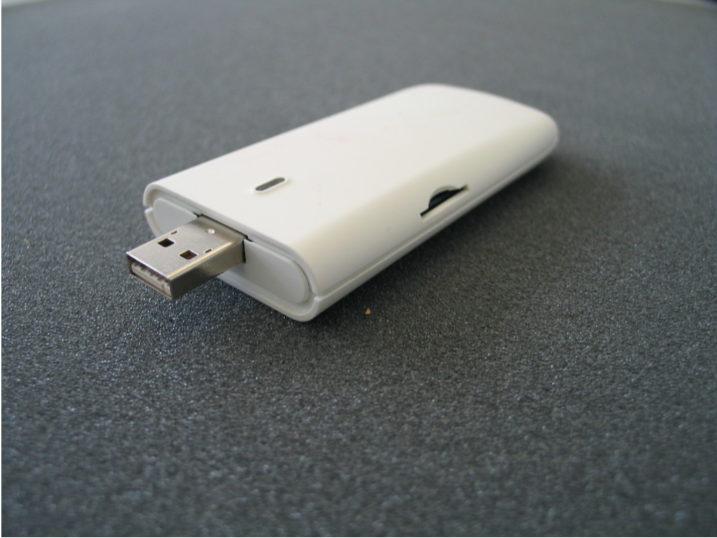
Photo 1: USB modem, top side, view to the USB connector, LED and SIM card interface
