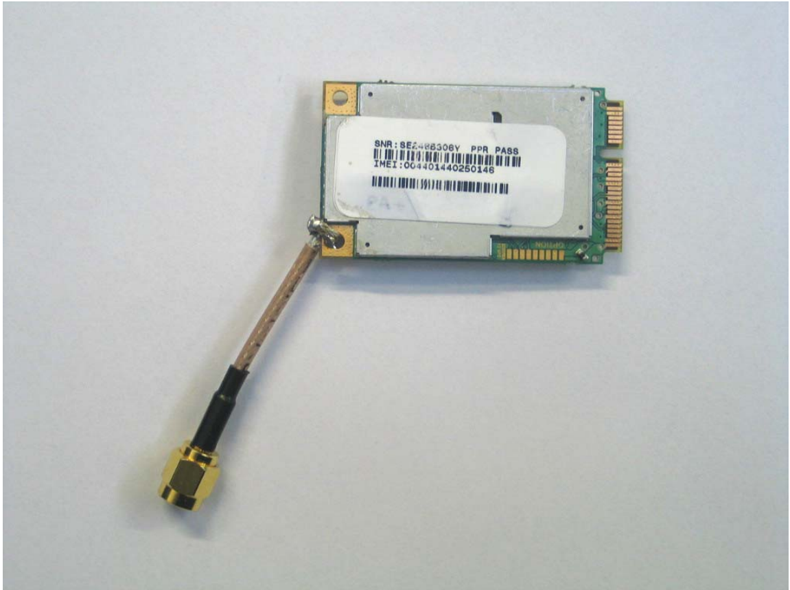
Photo 4: GSM/UMTS module (rear side)
